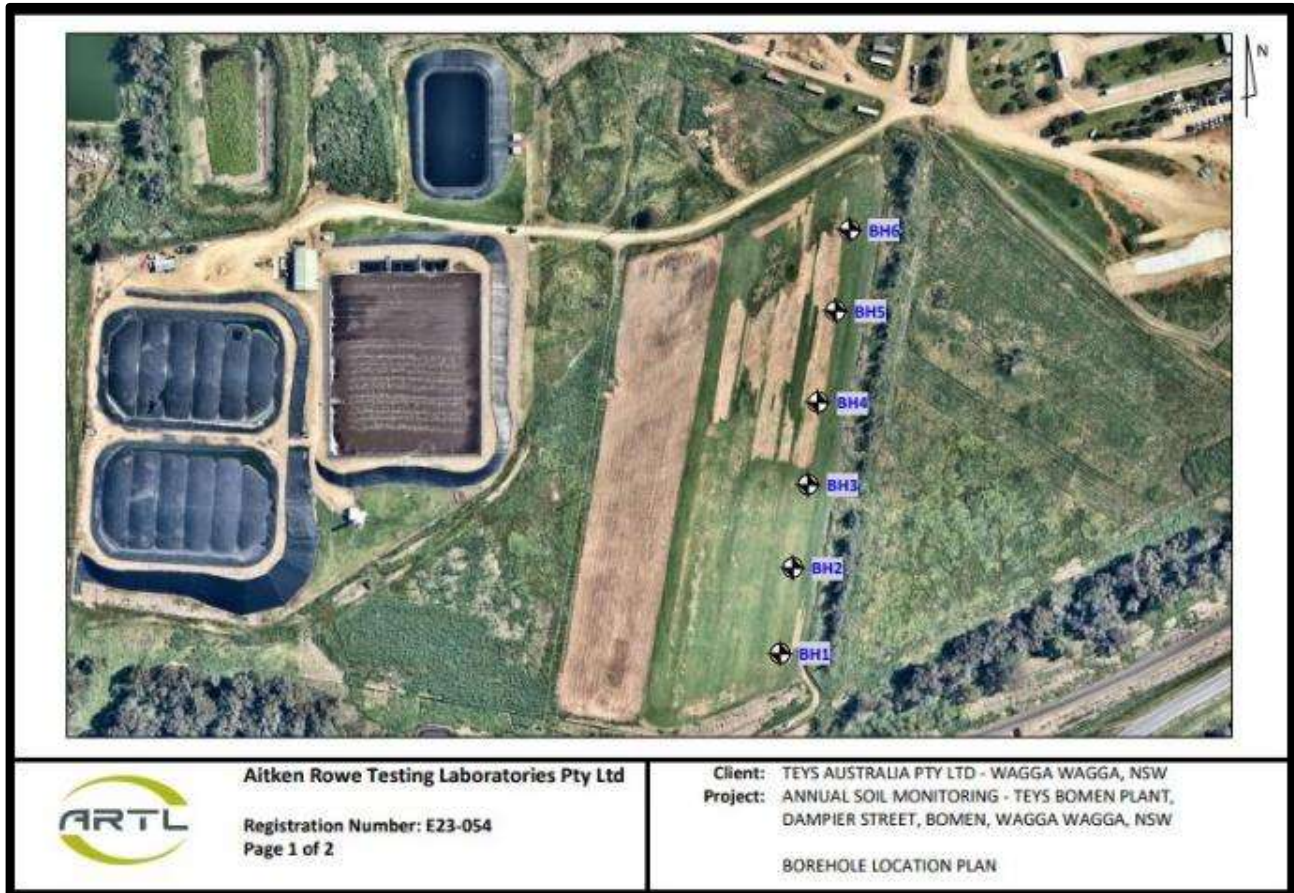
Figure 2: Monitoring Point EPA Identification Number 4 relating to soil testing. Soil test boreholes are drilled across the area for irrigation of treated process water to turf farming operations. Area is called CFA High.
