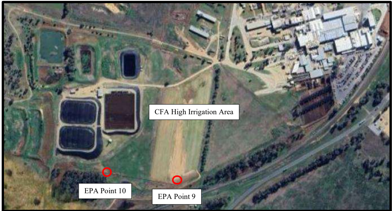
Figure 4: Monitoring Point EPA Identification Number 9 and 10. Groundwater testing piezometers (wells) downslope from CFA High irrigation and turf farming area.
