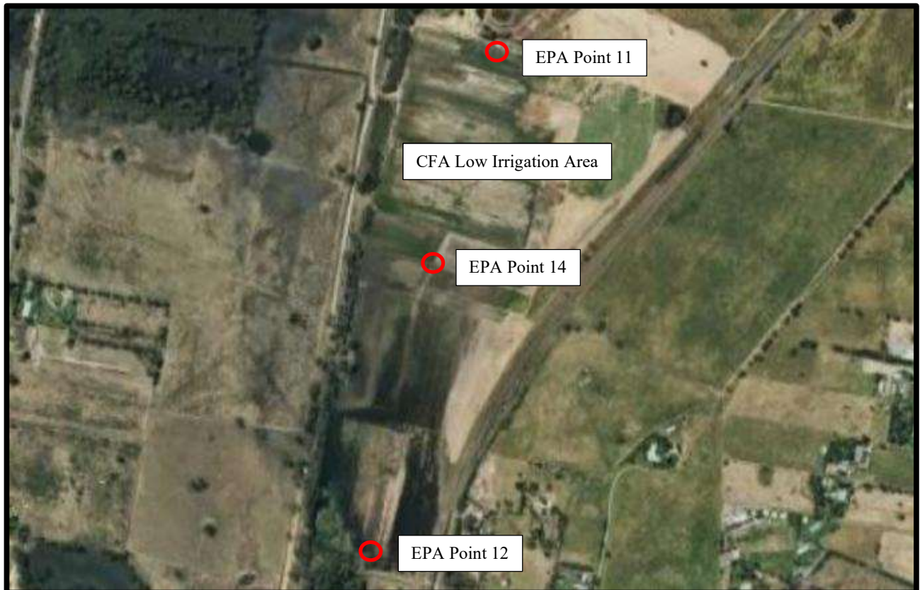
Figure 5: Monitoring Point EPA Identification Number 11, 12 and 14. Groundwater testing piezometers (wells) on CFA Low irrigation and turf farming area.
